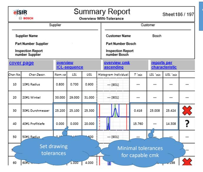
4. Overview table of all cmk values in ICL sequence – info of min tolerances for a capable characteristic
